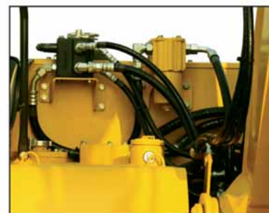
Shifting valve & expanded filter Shifting valve for breaker and crusher/common piping
